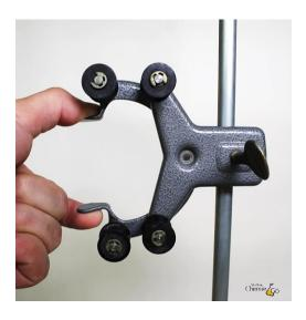
The burette clamp is opened using index finger and thumb.
