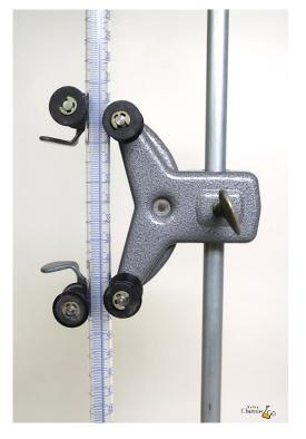
The burette is secured by positioning it between the rubber rollers. Subsequently, the clamp is carefully closed and the burette is ready for use. **Left:** A complete apparatus with burette and burette clamp.
